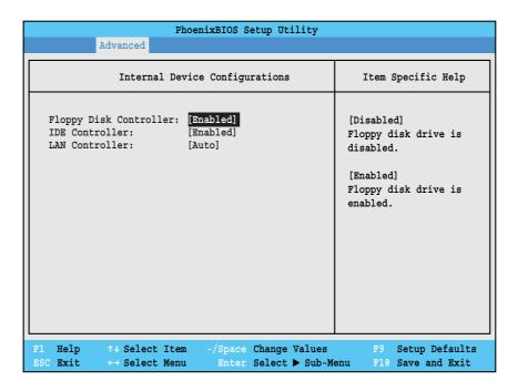
Figure 7. Internal Device Configurations Submenu
